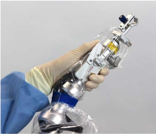
Pushing the free switch (which is colored gold) allows the arm to move freely.
