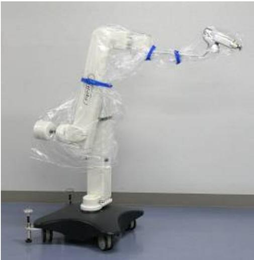
*After covering the device entirely with the drape, remove any slack by using blue tape, but without restricting the movement of the device.*
