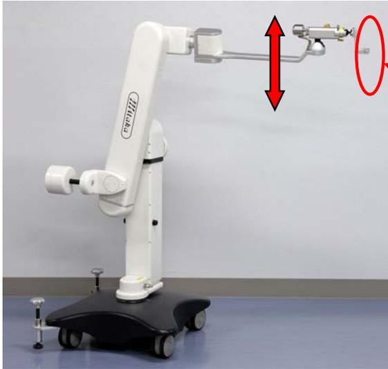
Balance the UniARM after attaching any instrument (endoscope, retractor).
